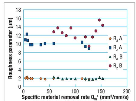
Fig 7 Variation in surface finish with increasing  $Q_w'$  for product A and B
