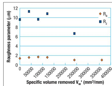
Fig 11 Change in surface roughness with cumulative volume ground for product A
