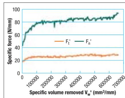
Fig 8 Variation in the specific forces for product A with increasing volume removed
