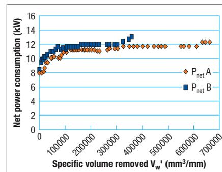
Fig 10 Change in net spindle power with cumulative volume of workpiece removed
